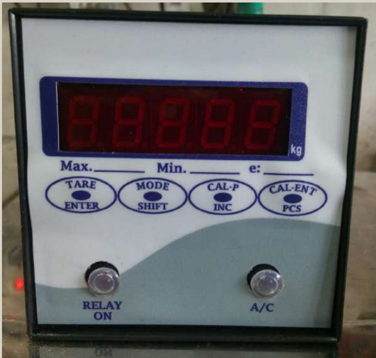
PLC INDICATOR 4-20 Ma OUTPUT INDICATOR
